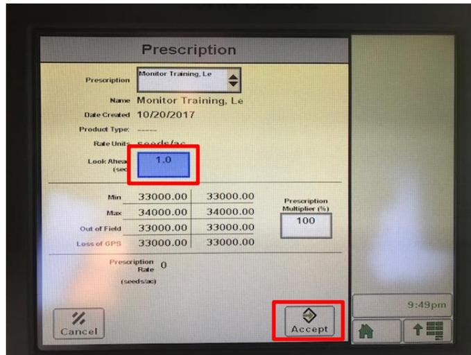
14. After accepting the Look Ahead timing, click on the Menu button on the bottom right corner and go to the **Planter** tab
